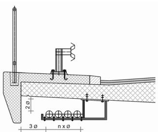
Fig. 9.1: Detail of fastening of installations below cantilever
