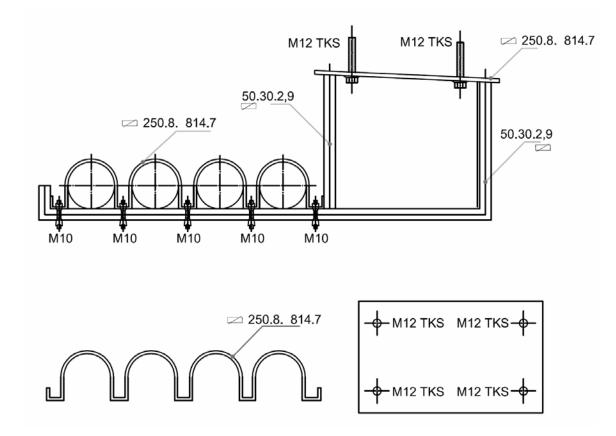
Fig. 9.2: Workshop drawing of suspension for four ducts
