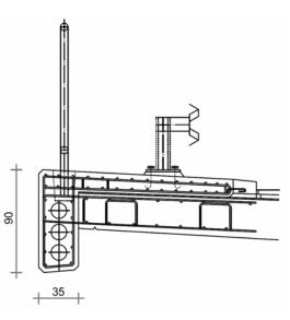
Fig.5.1a: 3 ducts of ∅ 125 mm in the edge beam
