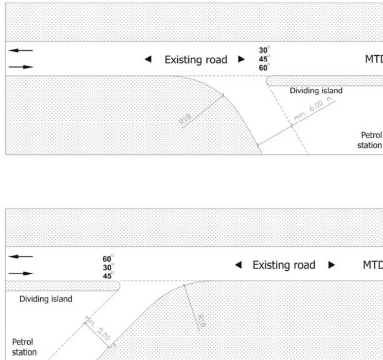
Figure 304: Diagonal inflow and outflow
