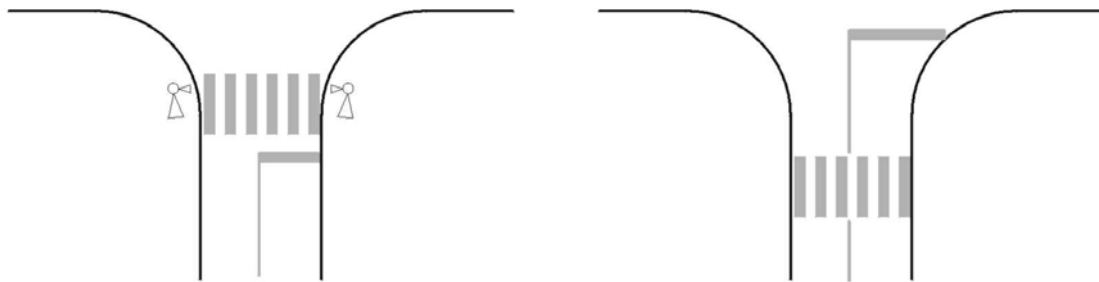
Figure 35: Location of a pedestrian crossing in traffic light controlled intersections and non-traffic light controlled intersections.
