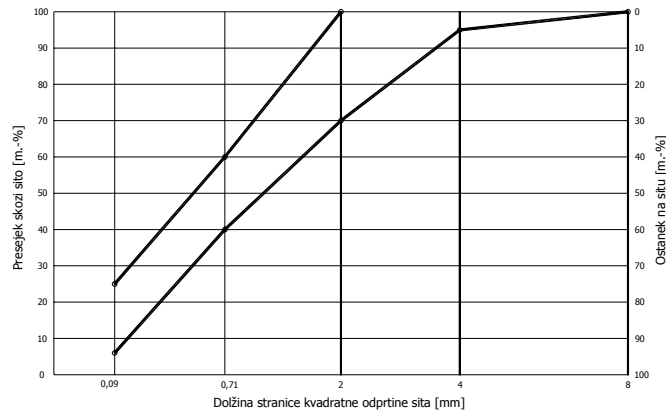
Fig. 3.33: Grading curve limits for mineral aggregate for asphalt mixtures for thin overlays TP 2h
