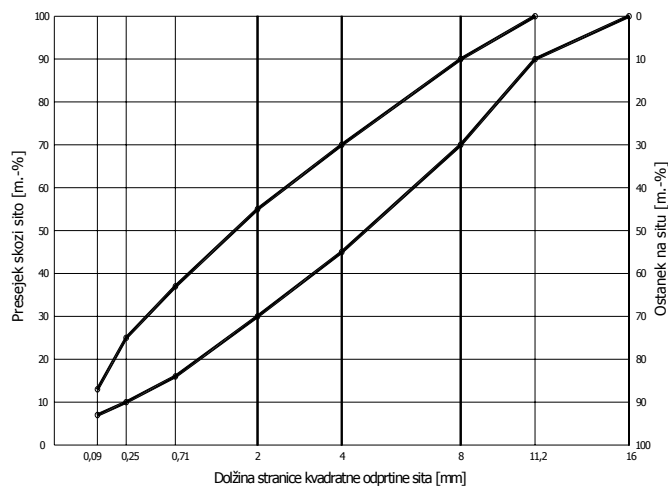
Fig. 3.18: Grading curve limits for mineral aggregate mixtures for bituminous concrete BC 11k, BC 11ks, and BC 11sk
